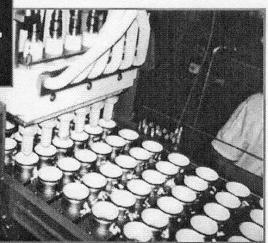
Introducing shoe change will not help if lines are not well CIP'd and contaminated condensation drops onto open product.
