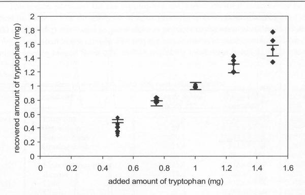
Figure 1 Recovery rate of tryptophan at different concentration (\$\phi\$ individual recovery rate, \$\I\pm 5\%\$ margin of error as limit of accuracy)
