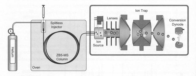
Figure 6 GC-ion trap system
