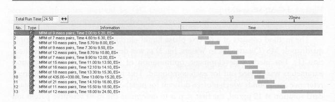
Figure 4 Multiple reaction monitoring in 13 acquisition groups
