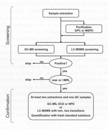
Figure 1 Flow chart of pesticides residue analysis
