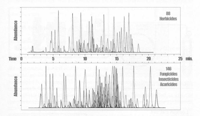
Figure 5 Chromatograms of standard mix at 0.1 µg/ml for herbicides, fungicides, insecticides and acaricides analysis
