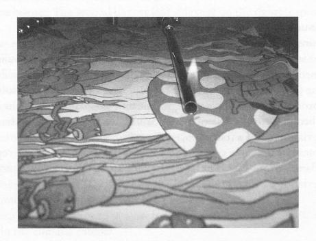
Picture 1 Duvet cover being tested with a small open flame according to EN 12952 parts 3 & 4
