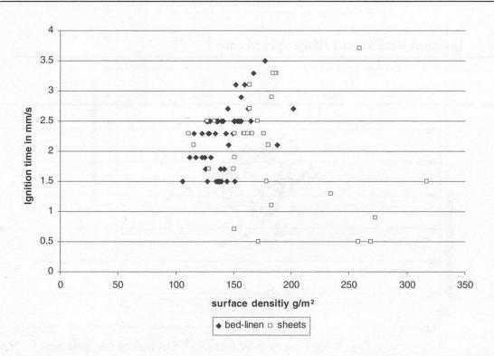
Figure 6 Ignition time versus surface density
