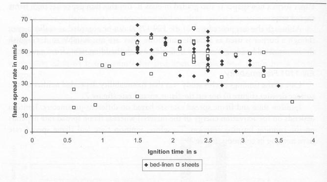
Figure 7 Ignition time versus flame spread rate
