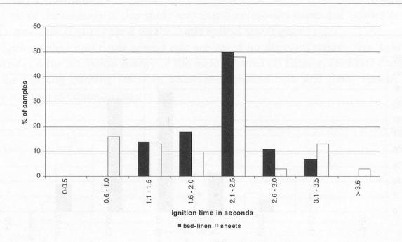
Figure 3 Ignition time according to ISO 6940 (bed-linen n=56, sheets n=31)
