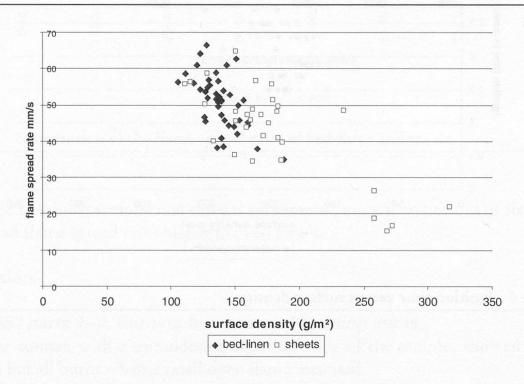
Figure 8 Flame spread rate versus surface density, EN 1102 (ISO 6941)
