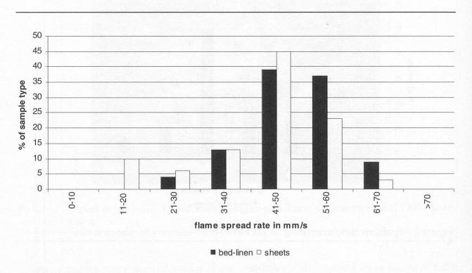
Figure 5 Distribution of the flame spread rates of bed-linen and sheets
