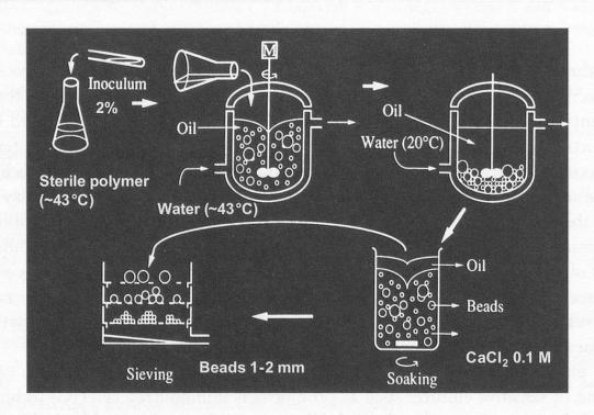
Figure 1 Double phase dispersion process for the production of spherical gel biocatalysts with immobilized viable cells (adapted from 8)
