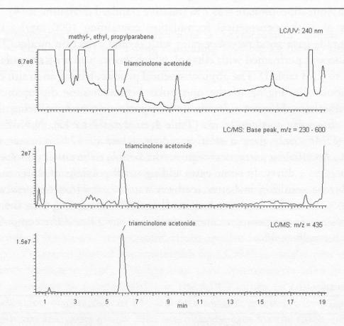
Figure 3 Comparison of HPLC/DAD with HPLC/APCI(+)- MS (base peak of full scan and m/z=435) of a phytocosmetic sample containing about 40 mg/kg triamcinolone acetonide
