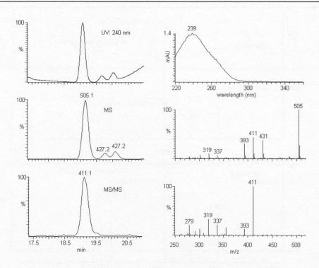
Figure 6 Comparison of HPLC/DAD with HPLC/APCI(+)- MS and HPLC/APCI(+)- MS/MS of a phytocosmetic sample containing about 600 mg/kg Betamethasone di propionate; LC/DAD notation: spectrum maximum (nm); LC/MS notation: m/z of most intense ion (base peak)
