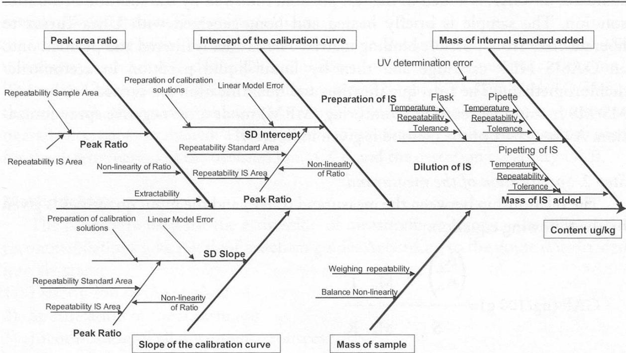
Figure 2 Cause and effect diagram of CAP analysis
