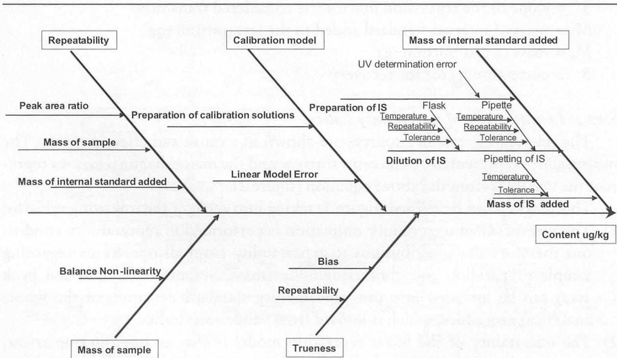
Figure 3 Refined cause and effect diagram
