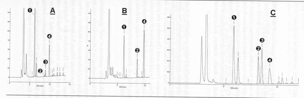
Figure 3 IE-Chromatogram of positive samples: A) calmars, B) shrimps and C) processed cheese, containing sodium monophosphate (5.9 min; peak 1), diphosphate (8.4 min; peak 2) and trimetaphosphate (8.7 min; peak 3), and triphosphate (9.7 min; peak 4) (for working conditions see text)
