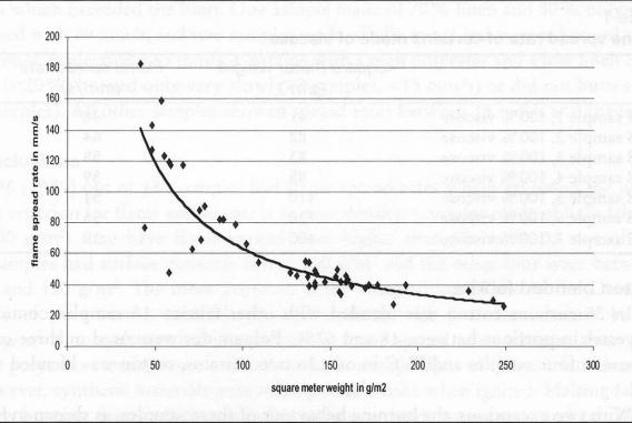
Figure 4 Cotton curtains: Flame spread rate versus surface density
