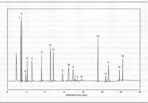
Figure 1 Chromatogram of a reference solution with detection at 300 nm (for peak identification, see table 1)
