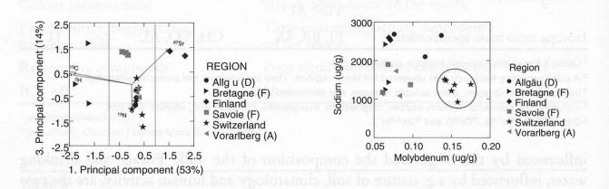
Figure 1 Principal component analysis of the parameters  $\delta^{13}$ C,  $\delta^{2}$ H,  $\delta^{15}$ N,  $\delta^{87}$ Sr. Clear separation of the groups "Finland", "Savoie" and "Bretagne" from the other regions
