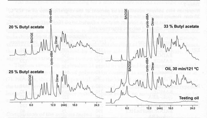
Figure 8 Migration from an epoxy/phenolic coating into oil and iso-octane containing 20-33 % n-butyl acetate (60° C/60 min): selectivity of oil and solvent substitutes is different (Y. Uematsu, unpublished results)
