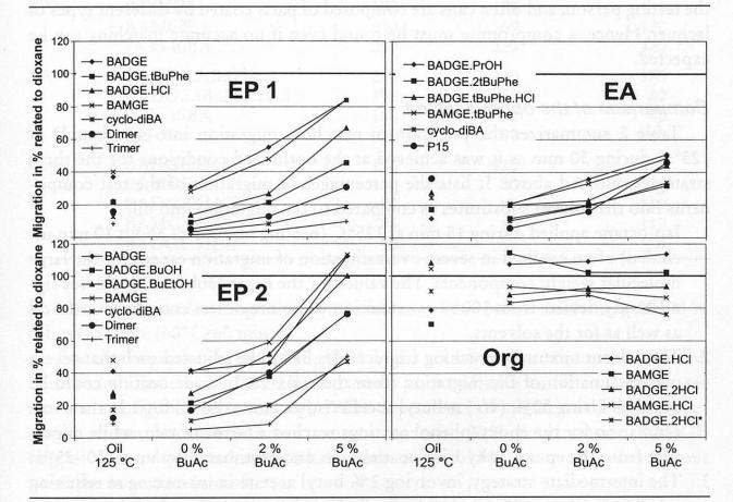
Figure 7 Migration into oil at 125°C/60 min (left) and into refluxing n-butyl acetate/iso-octane mixtures (v/v) (1 h)
