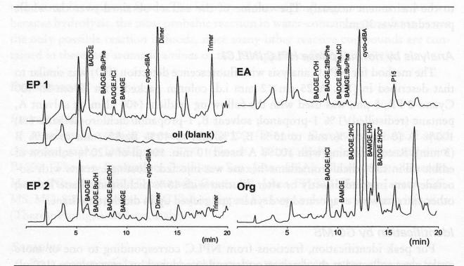
Figure 1 NPLC-FD chromatograms showing the migration into edible oil (125°C, 30 min) for the four coatings involved in the experiments. The components used for quantitating specific migration are assigned and listed in table 1. EP1 and EP2=epoxy/phenol coatings; EA=epoxy/anhydride; Org=organosol
