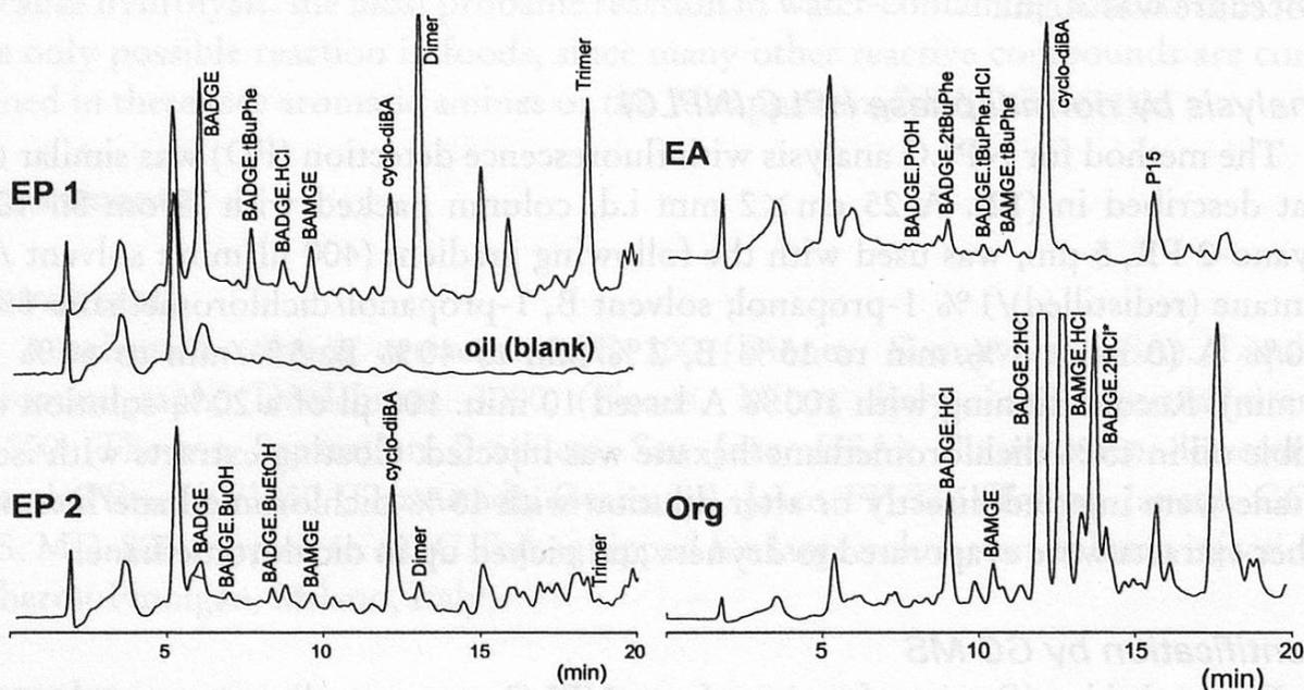
Figure 1 **NPLC-FD chromatograms showing the migration into edible oil (125°C, 30 min) for the four coatings involved in the experiments.** The components used for quantitating specific migration are assigned and listed in table 1. EP1 and EP2=epoxy/phenol coatings; EA=epoxy/anhydride; Org=organosol
