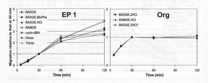
Figure 3 Dependence of migration into vegetable oil at 125°C on the duration of heating for the epoxy/phenol coating 1 (EP1) and the organosol (Org)
