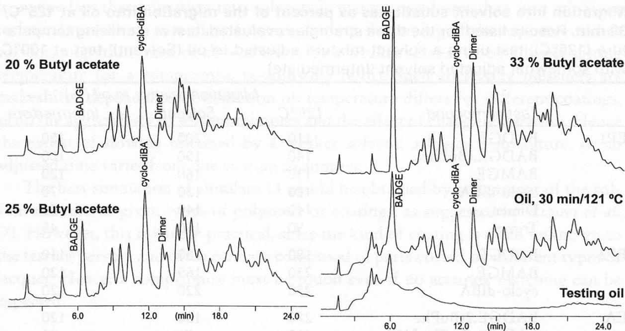
Figure 8 **Migration from an epoxy/phenolic coating into oil and iso-octane containing 20–33 % n-butyl acetate (60°C/60 min): selectivity of oil and solvent substitutes is different (Y. Uematsu, unpublished results)**
