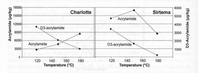
Figure 2 Acrylamide concentration and elimination of D<sub>3</sub>-acrylamide at various temperatures for potato of the cultivars Charlotte and Sirtema; concentrations referring to dry weight
