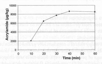
Figure 3 Acrylamide concentrations (referring to dry weight) after heating at 120°C for different duration
