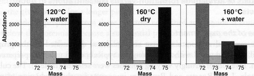
Figure 3 Signals of CI-MS for acrylamide and D<sub>3</sub>-acrylamide as obtained after heat treatment to 120 and 160°C with and without humidity
