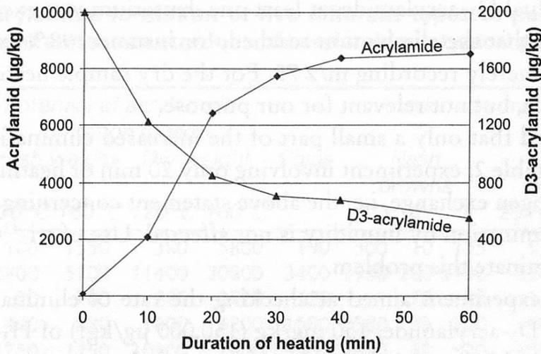
Figure 2 Acrylamide concentrations and D<sub>3</sub>-acrylamide elimination during heating of dried potato at 120°C
