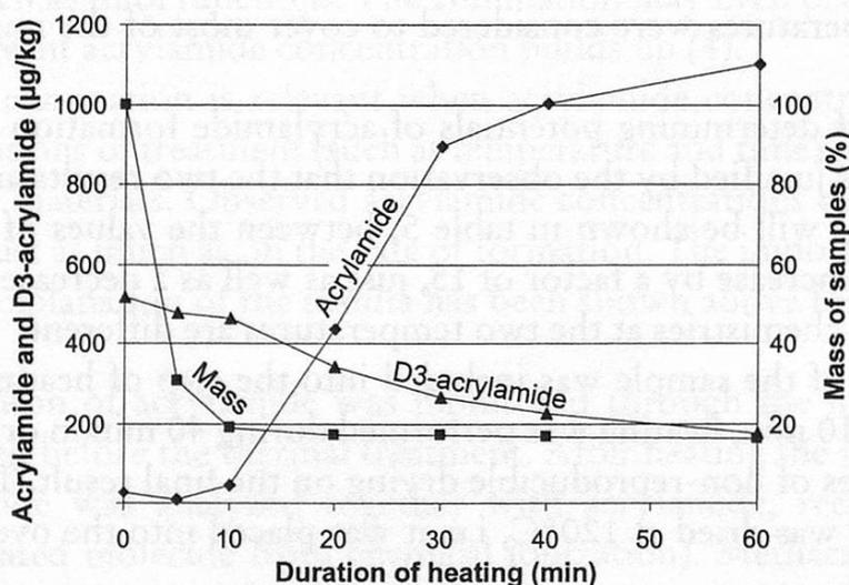
Figure 1 Concentrations of acrylamide and elimination of D<sub>3</sub>-acrylamide at 120°C, starting with fresh potato; mass of the samples after heating as percent of the fresh mass
