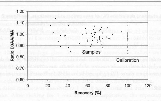
Figure 4 Area ratio of D<sub>3</sub>-acrylamide and methacrylamide for the calibration ("100% recovery") and the samples depending on the recovery over sample preparation as determined by the ratio of D<sub>3</sub>-acrylamide and butyramide
