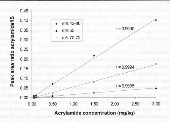
Figure 6 Linearity of the results for acrylamide
