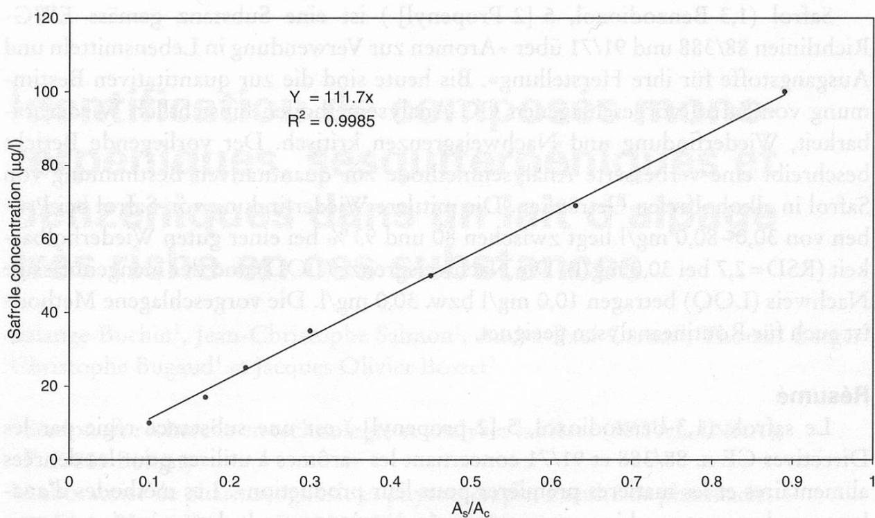
**Figure 1 Calibration curve for safrole quantitative determination over a linear concentration range of 10.0–100.0 µg/l obtained under the operating conditions described in the “Materials and methods” section**
