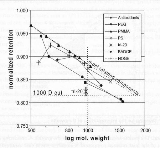
Figure 3 Normalized retention versus logarithmic molecular weight: results for the Phenogel 500 Å column with THF as mobile phase
