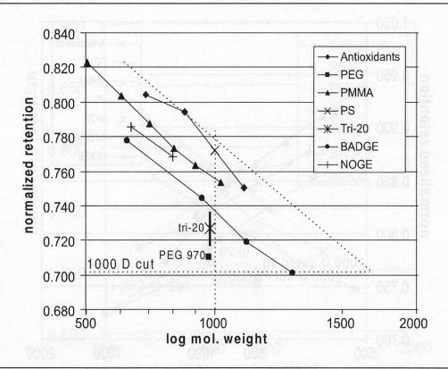
Figure 4 Normalized retention versus logarithmic molecular weight: results for the Phenogel 500 Å column with dichloromethane instead of THF as mobile phase
