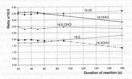
Figure 3 Control of side reactions during transesterification by treatment of ESBO-FAME.E.HCl with methoxide/methanol during the time indicated. Peak areas normalized on methyl stearate (18:0) as a component not expected to participate at possible reactions
