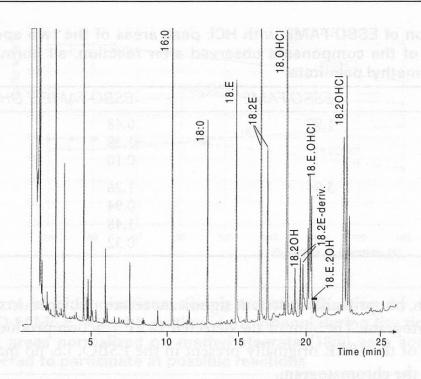
Figure 2 Gas chromatogram of acetylated ESBO-FAME.E.HCI. Peak identities, see table 1
