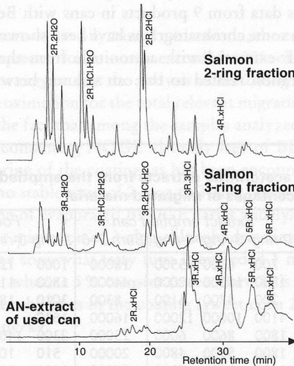
Figure 7 RPLC-FD chromatograms from canned salmon in water
