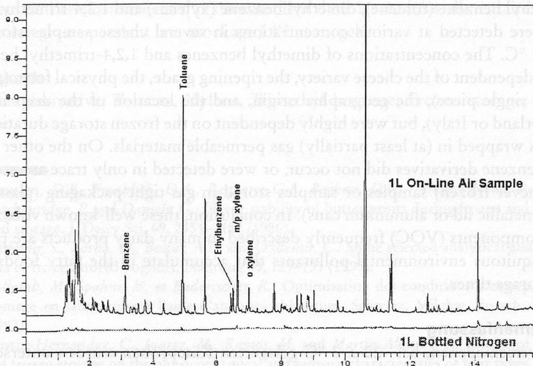
Figure 3 **Gas chromatogram of some benzene derivatives from surrounding air** (sampling in South Wales) **and nitrogen as reference sample** (reproduced with the kind permission of Markes International Ltd., Pontyclun, copyright by Hoppenstedt-Verlag, Darmstadt) (47)
