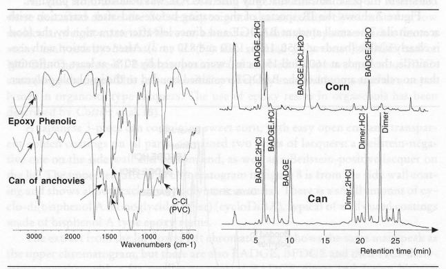
Figure 4 IR spectra from the internal surface of the extracted anchovy can and from a surface coated with an epoxy phenolic lacquer.
