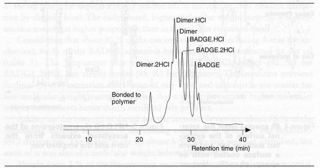
Figure 6 SEC-FD chromatogram of a hot dioxane extract of the sweet corn can, dissolving most of the polymer
