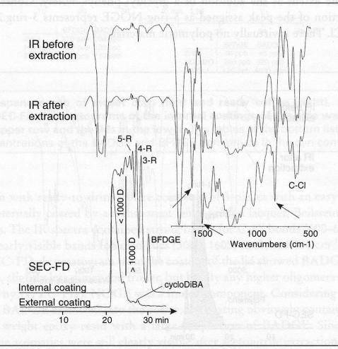
Figure 10 Can containing sausages: IR spectra of the internal coating of the easy open lid before and after extraction with acetonitrile (arrows on bands suggesting epoxy components). SEC-FD chromatograms of the lacquers from the internal and external lid surface
