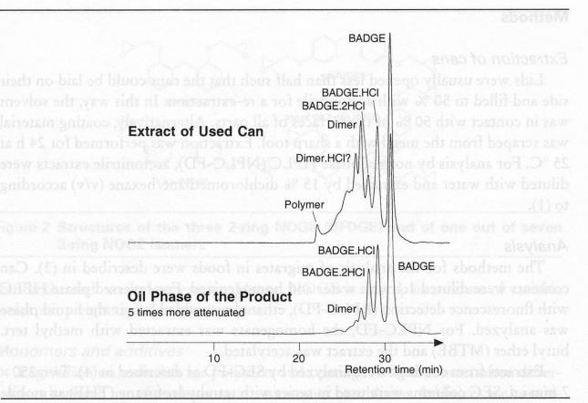
Figure 3 Anchovies in oil: SEC-FD chromatograms of the oil phase and of the extract from the emptied can
