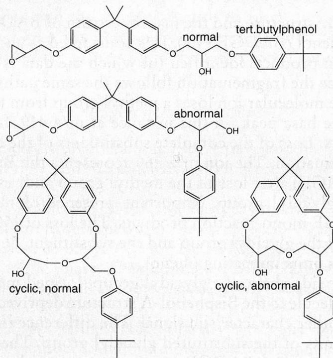
Fig. 2. Possible reaction products of tert. butylphenol with BADGE
