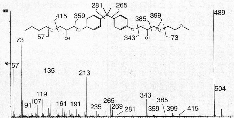
Fig. 4. Mass spectrum of BADGE reacted with butanol and 1-methoxy-2-propanol (BADGE.BuOH.MePrOH)
