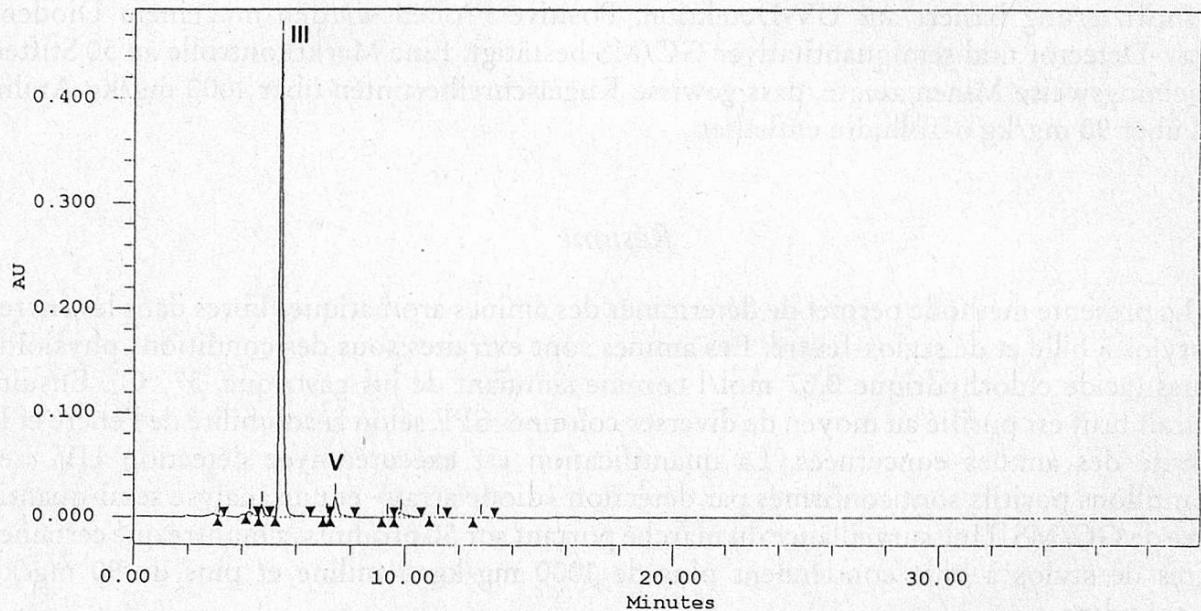
Fig. 3b. HPLC run of eluate 1 of a ballpoint pen containing aniline (III) and o-toluidine (V)
