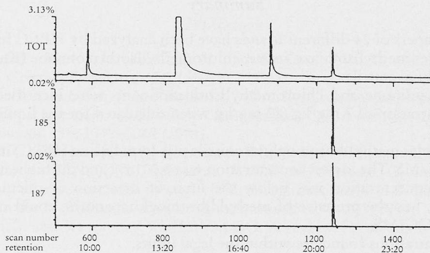
Fig. 2. GC/MS chromatogram of a sample moist toilet paper (nr 16). Chromatograms of the total of all ions measured (tot) and of the ions at masses 185 and 187. Conditions as described in the text
