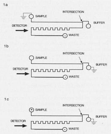
Fig. 1. Layout of a glass device with different potential settings: for injection (a), for separation (b), and for mixing of two solutions (c). Most channels are 10 μm deep. The channel lengths (width) are as follows: sample reservoir to intersection, 4.5 cm (30 μm wide); buffer reservoir to intersection, 0.8 cm (30 μm wide); intersection to waste reservoir, 9.0 cm (30 μm wide) and 2.3 cm (220 μm wide)
