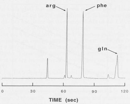
Fig. 3. Electropherogram of 3 FITC-labelled amino acids in pH 9.2 carbonate buffer. The peaks were identified by injecting each component separately. (Reprinted with permission from (7). © 1993 American Chemical Society)
