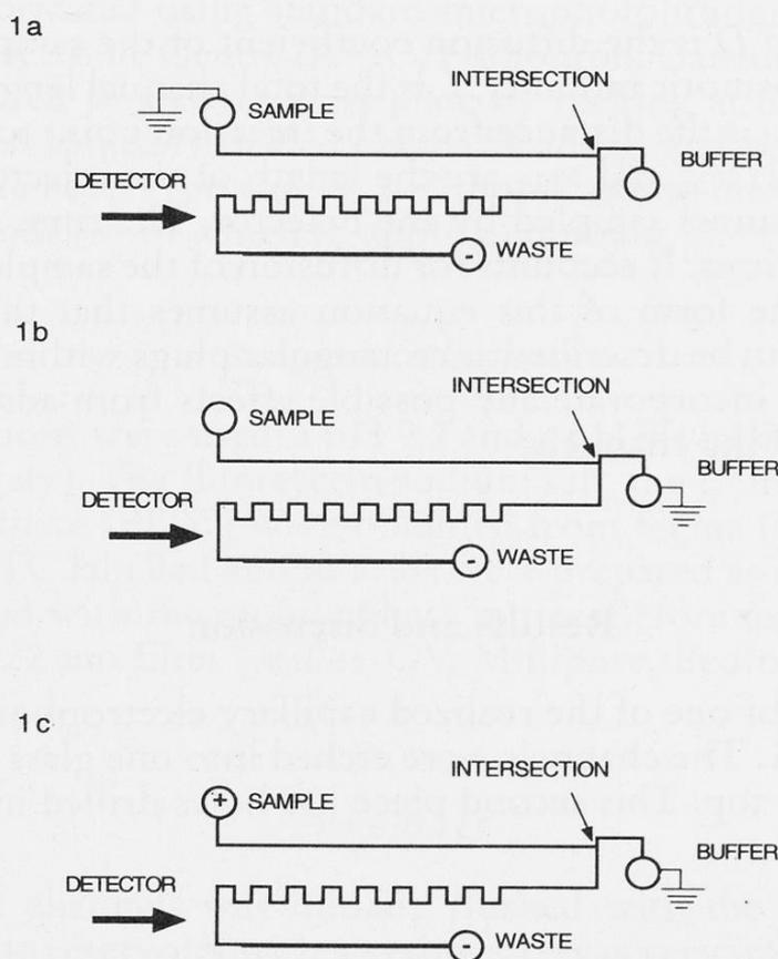
Fig. 1. Layout of a glass device with different potential settings: for injection (a), for separation (b), and for mixing of two solutions (c). Most channels are 10  $\mu$ m deep. The channel lengths (width) are as follows: sample reservoir to intersection, 4.5 cm (30  $\mu$ m wide); buffer reservoir to intersection, 0.8 cm (30  $\mu$ m wide); intersection to waste reservoir, 9.0 cm (30  $\mu$ m wide) and 2.3 cm (220  $\mu$ m wide)
