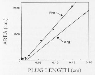
Fig. 4. Peak area as a function of the calculated plug length for Arg and Phe. (Reprinted with permission from (7). © 1993 American Chemical Society)
