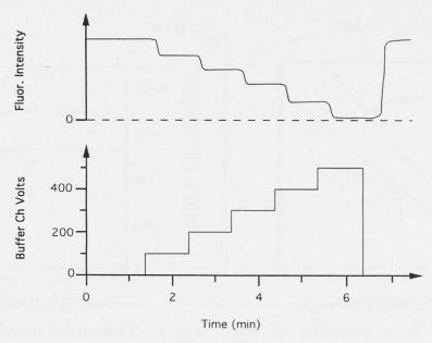
Fluorescence intensity downstream of the T-intersection is shown as a function of time, while the potential on the buffer channel was increased with time
