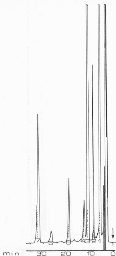
Fig. 5. HPLC sample 20 (black) 1 = Ascorbic acid 5 = 24DAA = 0.20 % 2 = RES = 0.2% 6 = Unknown 3 = 25TDA = 2.93% 7 = Unknown 4 = Unknown
