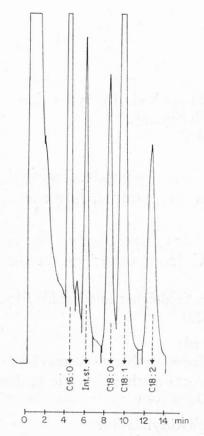
Fig. 2. GLC of methylesters of ovo phosphatidylcholine fatti acids TLC-GLC determination of PC in a fresh egg yolk sample
