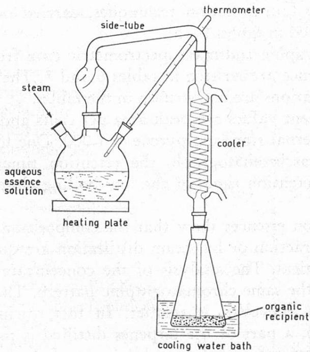
Fig. 3. Apparatus for the isolation of volatile compounds from essences by steam distillation
