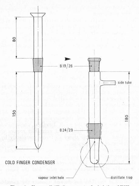
Figure 1. Vacuum distillation apparatus for isolation of ECH
