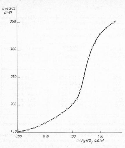
Fig. 3. Titration curve of 25 ml of the absorbing alkaline solution containing  $4.7 \times 10^{-4}$  M of chloride (5 ppm as coffee content); The solution was 25 % alcoholic, acidified with HNO<sub>3</sub> and cooled to O  $^{\circ}$  C before titration.
