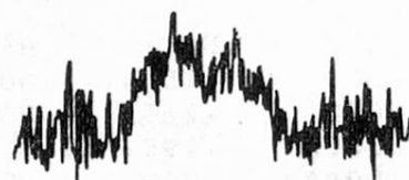
SIGNAL ARRIVING AT THE COMPUTER WITHOUT EXTENSIVE TRANSMISSION LINE CONDITIONING
