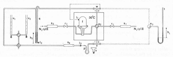
Fig. 3. Arrangement for concentrating food volatiles permeated through packaging foils
