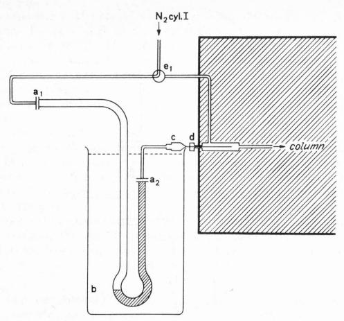
Fig. 1. Arrangement for sample introduction by pre-column
