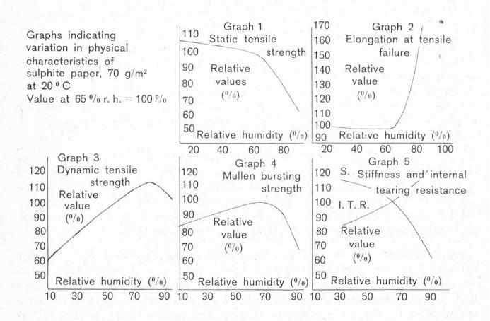
It is important to perform these tests under use conditions. Thus tensile properties of fibrous materials vary with relative humidity as is shown in Graphs 1 to 5. These show a number of interesting features. For instance although static tensile strength falls as relative humidity increases, elongation prior to failure increases and thus the energy required to cause a break (measured by Dynamic Tensile Strength) increases to a maximum at about 80 % r. h.
