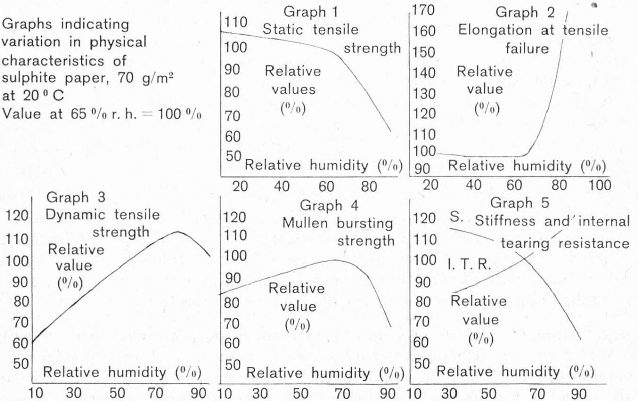
It is important to perform these tests under use conditions. Thus tensile properties of fibrous materials vary with relative humidity as is shown in Graphs 1 to 5. These show a number of interesting features. For instance although static tensile strength falls as relative humidity increases, elongation prior to failure increases and thus the energy required to cause a break (measured by Dynamic Tensile Strength) increases to a maximum at about 80 % r. h.
