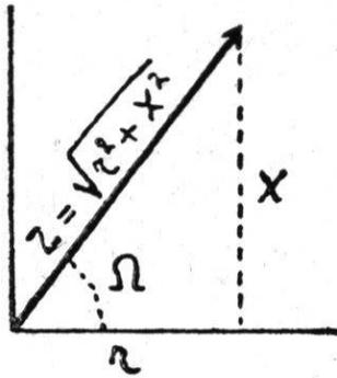
$$\begin{aligned} r &= z \cos \omega \\ x &= z \sin \omega \\ \operatorname{tg} \omega &= \frac{x}{r} \end{aligned}$$
