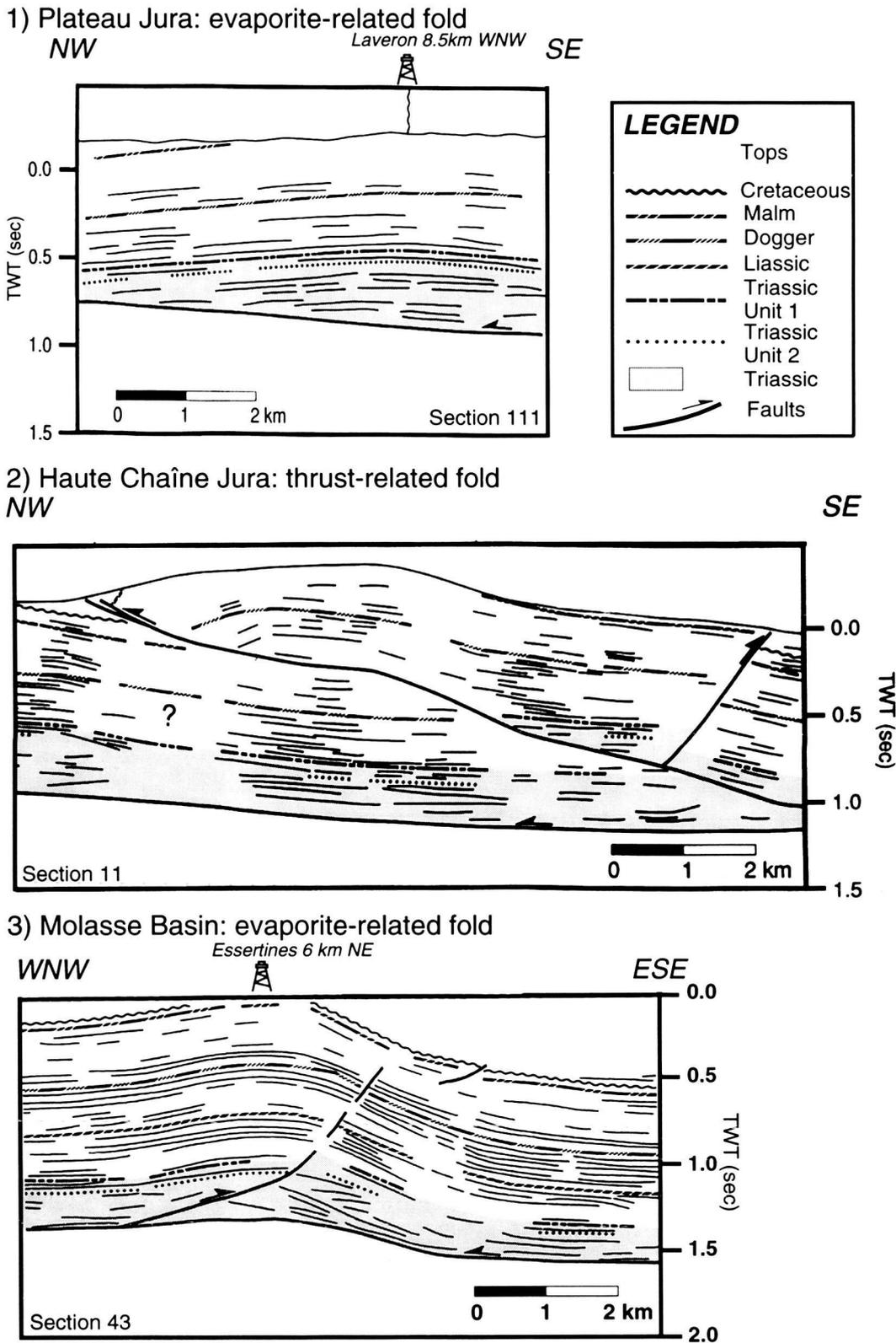
**Figure 5.3:** Line drawings of examples of typical fold structures in the Jura and the Molasse Basin (example numbers refer to Figure 3.1). Horizontal scale is in meters, whereas vertical scale is in seconds (two way travel time). Triassic Unit 2 is highlighted in gray. Examples 1 and 3 show low amplitude evaporite-related folds, whereas example 2 presents a high amplitude thrust-related fold. Modified from SOMMARUGA (1995).
