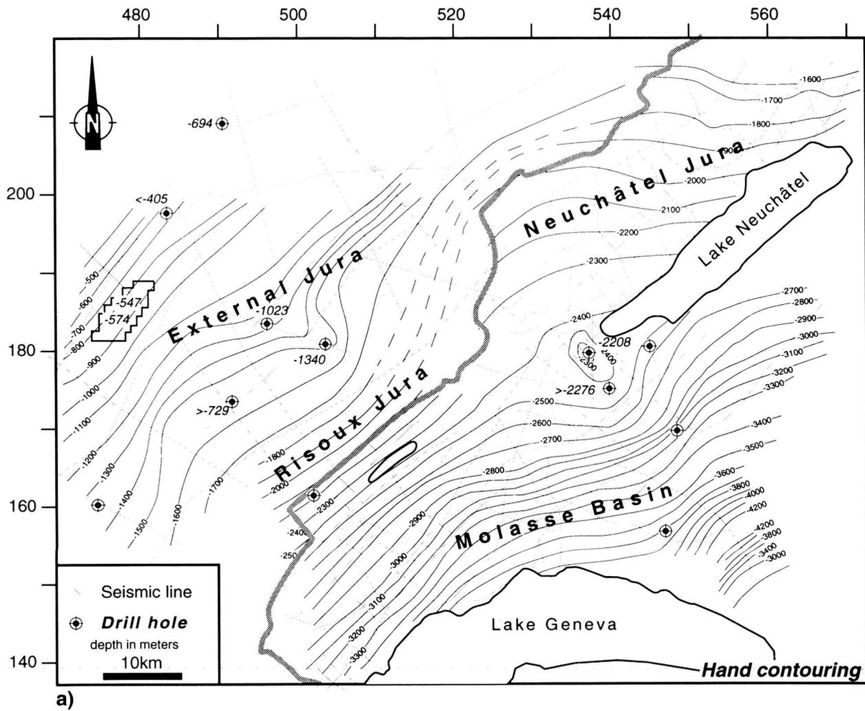
**Figure 5.1 (pages 142, 143):** Map of the depth to top basement in the central Jura and western Molasse Basin. Depths are in meters with reference to the sea level. Depths next to drill holes correspond to top basement depth from drill hole data. Minimal depths (>...) are from drill holes which ended within the Triassic layers. No depth indication is given for drill holes which did not reach the Triassic. Coordinates (in km) are according to the Swiss national geographical coordinate system.
