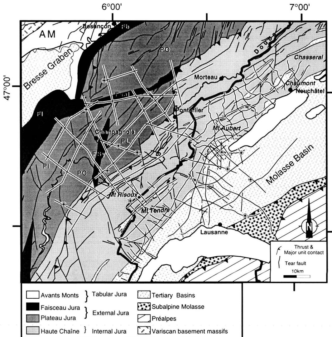
**Figure 4.1:** Seismic grid located on a tectonic sketch of the central Jura and the western Molasse Basin. Legend: AM = Avants-Monts; Fb = Faisceau bisontin; Fl = Faisceau lédonien; Fsal = Faisceau salinois; FSy = Faisceau de Syam; PC = Plateau de Champagnole; PL = Plateau de Levier; Pl = Plateau lédonien; PO = Plateau d'Ornans.
