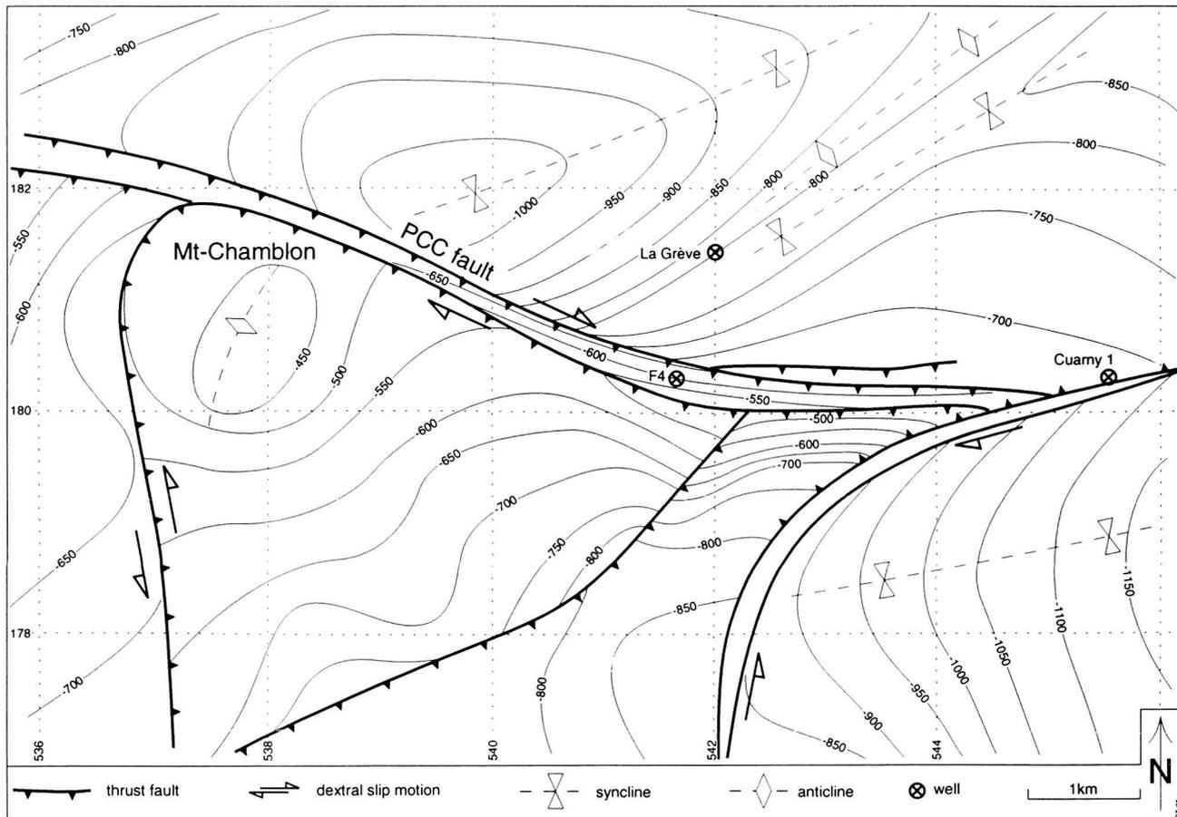
**Figure 4.19:** Contour map of the top Dogger in the Yverdon-Treycovagnes area, western Molasse Basin. Depths are in meters, below sea level. Numbers on the side and bottom are in kilometers that relate to the Swiss national geographical coordinate system. Modified from MURALT *et al.* (1997).
