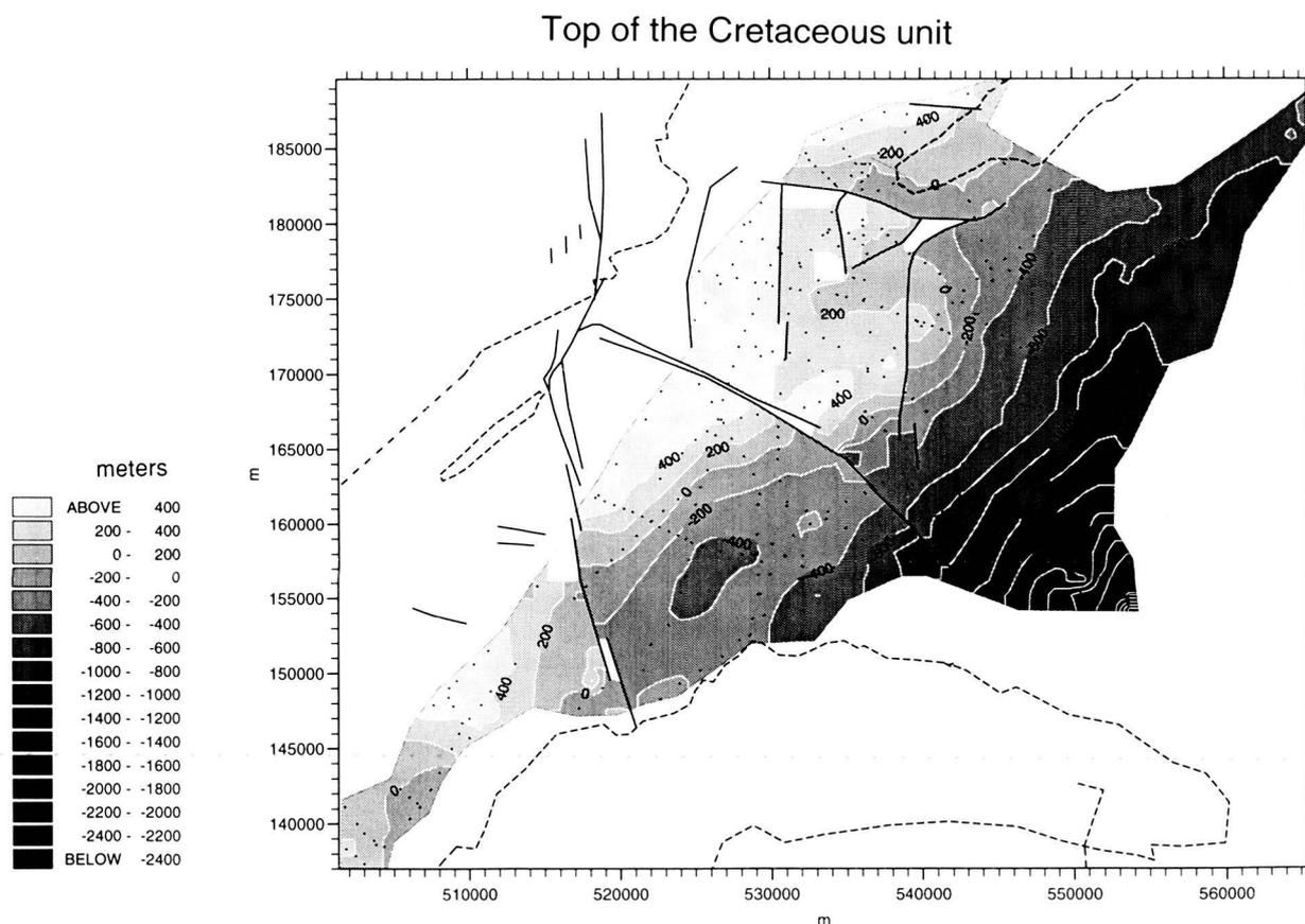
**Figure 4.11:** Contour map of the top Cretaceous unit in the western Molasse Basin. Depths are in meters. Black dots are shotpoints used for depth control of contour map. Note that blank areas and tight closed circles are computer-related artefacts in areas of sparse control. Numbers on the side and bottom are in meters, that relate to the Swiss national geographical coordinate system. Lakes Geneva and Neuchâtel are outlined for general reference.
