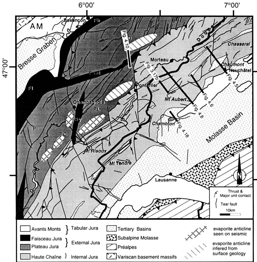
**Figure 4.9:** Tectonic sketch of the Jura and Molasse Basin with location of the evaporite-related anticlines of the external Jura. Geological cross-sections presented in this work are also located in this Figure. Legend: AM = Avants-Monts; Fb = Faisceau bisontin; Fl = Faisceau lédonien; Fsal = Faisceau salinois; FSy = Faisceau de Syam; PC = Plateau de Champagnole; PL = Plateau de Levier; Pl = Plateau lédonien; PO = Plateau d’Ornans.
