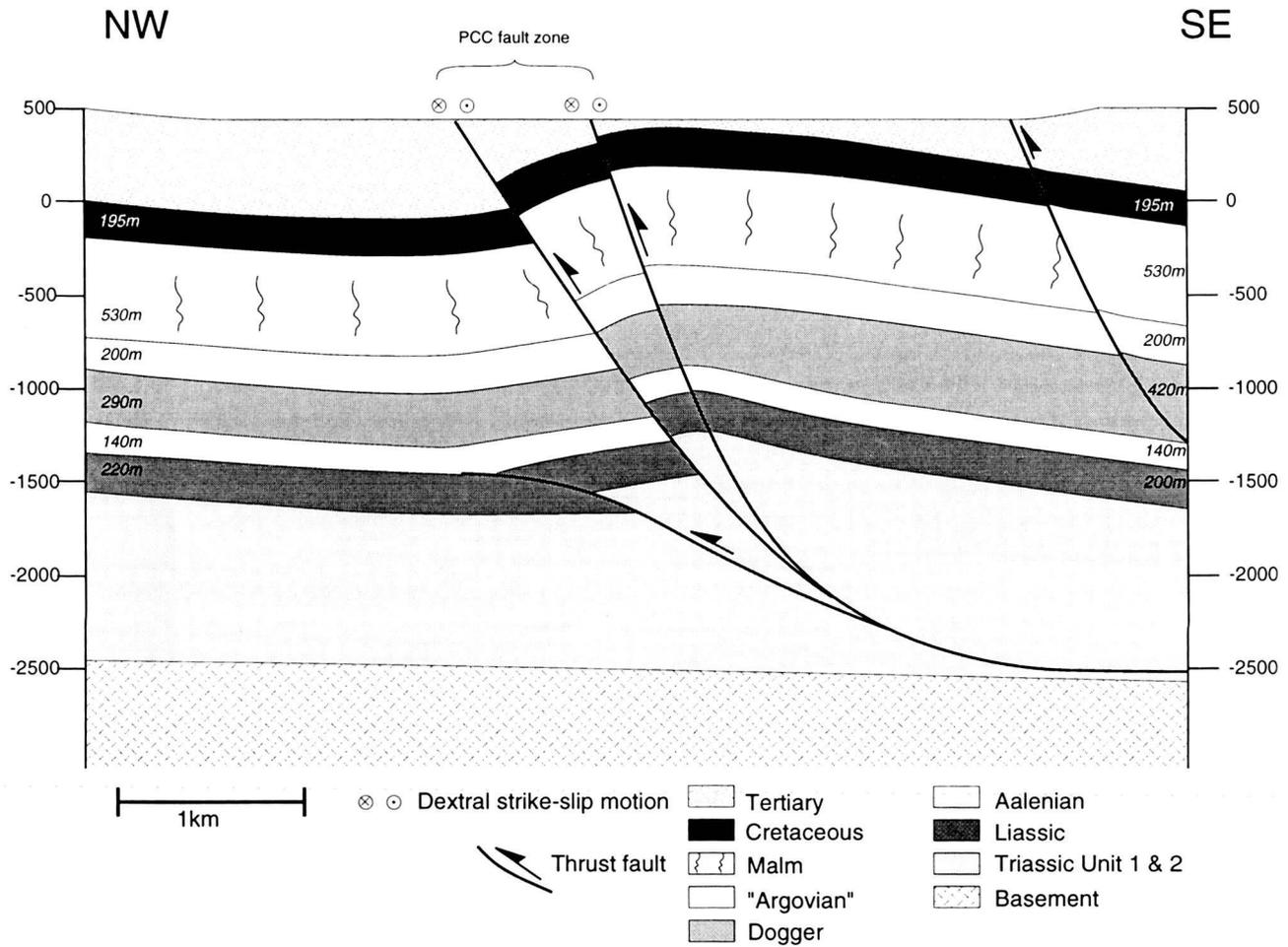
**Figure 4.18:** Geological cross-section oriented NW-SE based on surface geological data and completed at depth with information from seismic Section 25, Section 27 (Panel 5) and Section 38 (Panel 6). This geological section crosses the Chamblon hill (for location see Figs. 4.3 and 4.9). Modified from MURALT *et al.* (1997).
