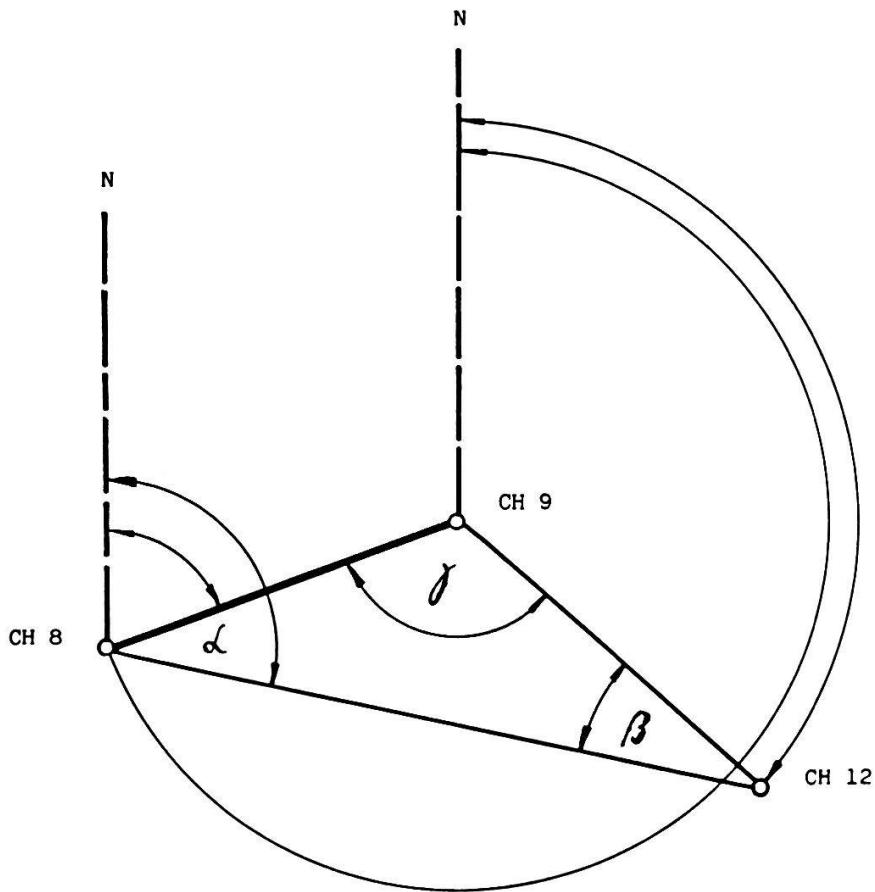
$$\text{Winkel } \gamma = 248^\circ 48' 11,8'' - 131^\circ 58' 29,79'' = \underline{116^\circ 49' 42''}$$
