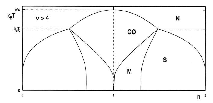
Figure 1.2: (n,T)-phase diagram for the canonical ensemble (thermodynamic limit at particle density  $n \in ]0,2[$  with suppressed fluctuations [8]).
