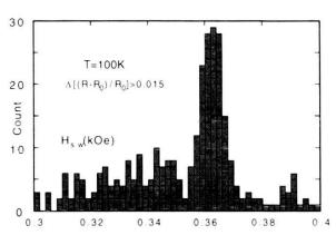
Fig. 3. Histograms of the switching fields, measured at 6 and 100 K.
