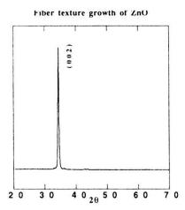
Figures show the equilibrium growth of ZnO and the corresponding surface morphology. The film was grown by the method of sputtering. Here the c-axis of the hexagonal wurtzite structure of the ZnO film is perpendicular to the substrate. The surface mobility, along with the anisotropic reaction of water vapour lead to the growth of surface with hexagons.
