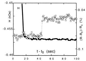
Fig. 2 Left graph: zoom of the central part of a longitudinal AMR hysteresis loop. Right graph: magnetoresistance ratio versus time. Shaded line: applied field versus time, showing that the step of the AMR can spontaneously occur within our filed peak to peak noise of 0.5 Oe. The field is fixed at -0.457 Oe.
