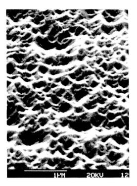
The surface mobility could be increased in several ways. In RF sputtering, the RF power plays an important role in making surface textured ZnO films. In CVD, the substrate temperature and the ratio of reacting gases play the decisive role with respect to the surface morphology. With these conditions we could succeed in obtaining 'surface textured' ZnO films with unique surface morphologies.
