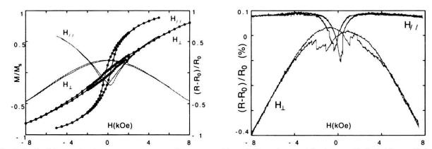
Fig.1 Left: Magnetization measurement of an assembly of Co wires, with the applied field parallel or perpendicular to the wire axis. Shaded lines: typical AMR curve shape deduced from an hypothesis of uniform rotation of the magnetization. Right: magnetoresistance AMR curves, for the two field orientations.
