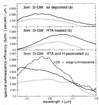
Fig.2: Comparison of PL spectra (300K) for a 3nm wide single quantum well embedded in  $SiN_x$  cladding layers (a-c) and a  $SiN_x$  film deposited on Si substrate (d). a) as deposited; b) after RTA at 1100°C, c) after hydrogen passivation. Solid lines: E-field of exciting and PL light perpendicular to the QW layer. Dotted lines: E-field parallel to QW.
