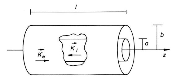
Figure 3: Two concentrical cylinders making a coaxial cable, with opposite currents flowing along the axial direction.
