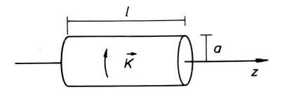
Figure 2: Cylinder with surface poloidal current density.
