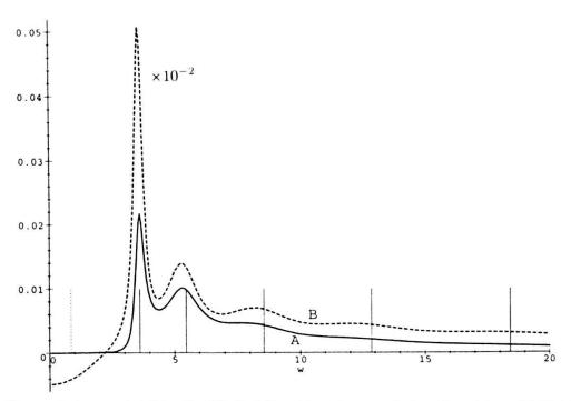
Figure 1: Transmission probability  $\mathcal{P}_{\rm tr}(E)$  (full line A) and transmission time delay  $\tau^{\rm tr}(E)$  (dashed line B), as a function of frequency  $\omega$ . Time delay is scaled by a factor  $10^{-2}$ . The vertical dotted line corresponds to  $\omega_{\rm BL} = 1/\tau_{\rm BL}$ . The other full vertical lines correspond to frequencies such that  $E + \hbar \omega$  is equal to a resonance energy of the static transmission probability.
