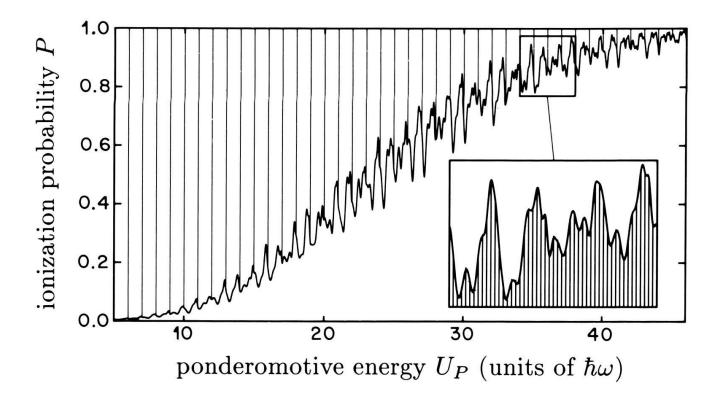
Fig.1 Ionization probability P as a function of  $\mu^2/2\omega^3$  for  $\omega_0/\omega = 10$  after 10 optical cycles.
