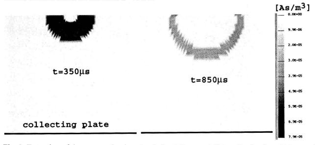
Fig. 2: Extension of the propagating ion cloud after 350  $\mu$ s and 850  $\mu$ s for the short 300  $\mu$ s pulse. The conditions are identical to those of Fig. 1.
