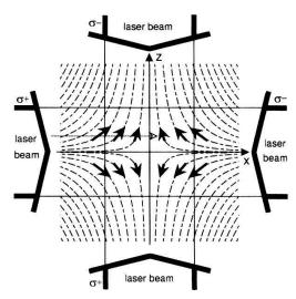
FIG. 3. The anti Helmholtz coils produce a spatially varying magnetic field in the trap. For an atom moving displaced from the axis the circular polarised laser beams drive  $\Delta m = 0, \pm 1$  transitions in the basis defined by the magnetic field.
