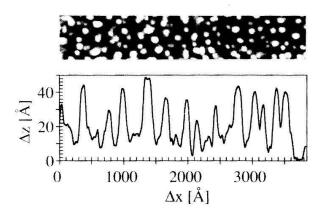
Fig.2: a) STM topograph after plasma cleaning, b) Cross section showing the surface roughness (Tip bias  $V_t=3V$ , tunneling current  $I_t=0.5nA$ ),.
