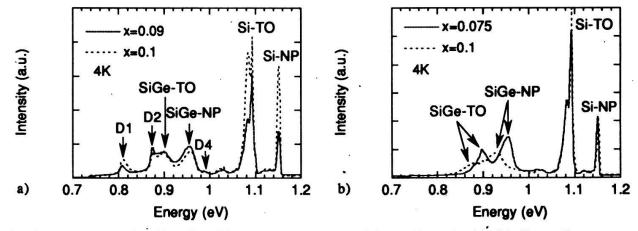
Fig. 2 PL Spectra for Si<sub>1-x</sub>Ge<sub>x</sub>/Si structures grown without (a) and with (b) C<sub>3</sub>H<sub>8</sub> flux.
