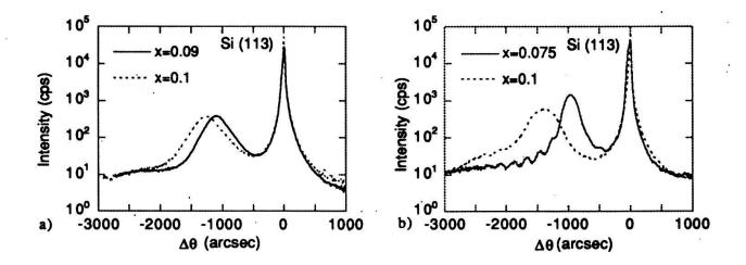
Fig. 1 XRD Spectra for Si<sub>1-x</sub>Ge<sub>x</sub>/Si structures grown without (a) and with (b) C<sub>3</sub>H<sub>8</sub> flux.
