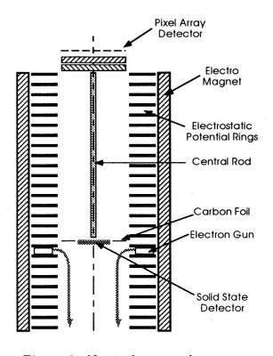
Figure 2: Neutral gas analyzer
