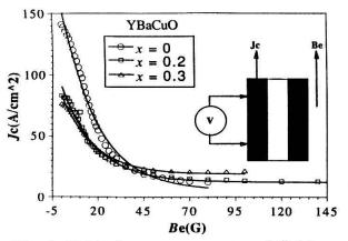
Fig. 1 Critical current vs. external field
