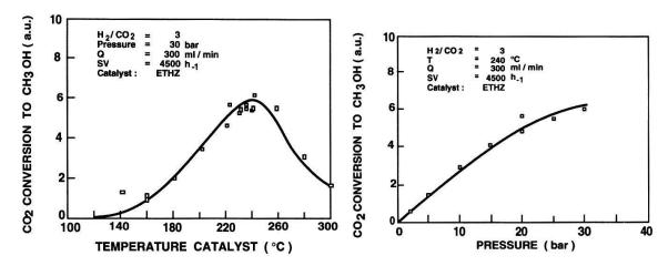
Fig. 1 Conversion of CO<sub>2</sub> to methanol as a function of temperature
