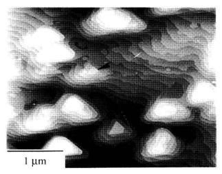
Fig.3: Large scale STM scan taken from a Si-buffer grown at  $700^{\circ}$ C showing step pinning at stacking faults (indicated by arrow) and screw dislocations. (V<sub>t</sub>=-2V, I<sub>t</sub>=0.5nA),.
