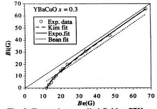
Fig. 2 Trapped vs. applied field at 77K
