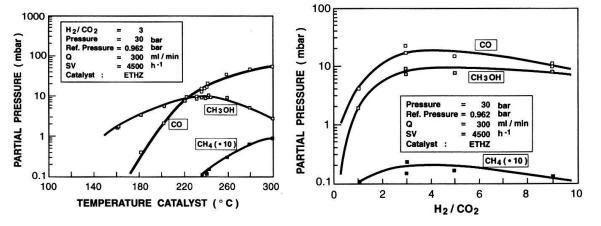
Fig. 3 Conversion of CO<sub>2</sub> to CO, CH<sub>4</sub>, CH<sub>3</sub>O<sub>4</sub> as a function of temperature
