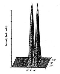
Fig. 1: Far-field intensity pattern of diode-laser emission
