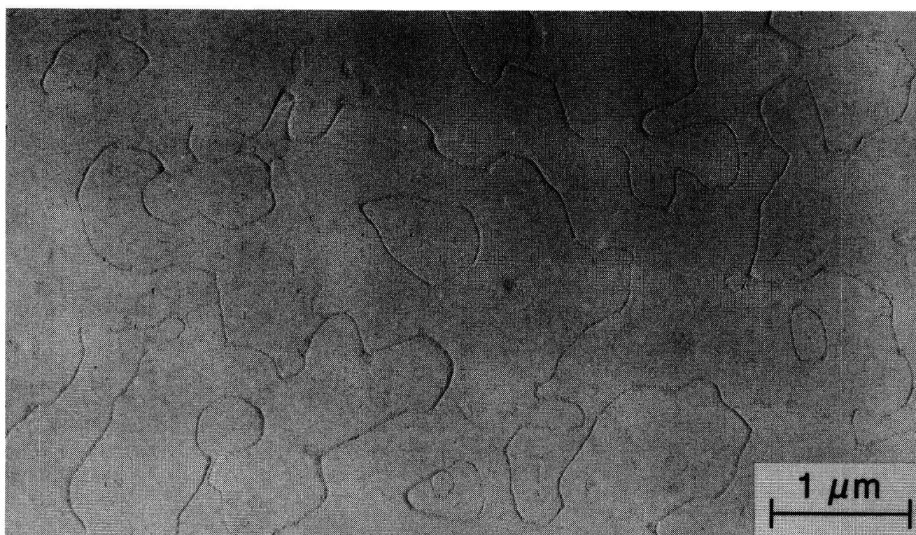
Fig. 1: Twin domains on a 200 nm thick AgBr film vapour-deposited on mica at room temperature. TEM replica technique.
