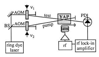
Figure 2: Experimental setup: BS = beam splitter, AOM = acousto-optic modulator, rf = radio-frequency synthesizer, PD = photodiode.
