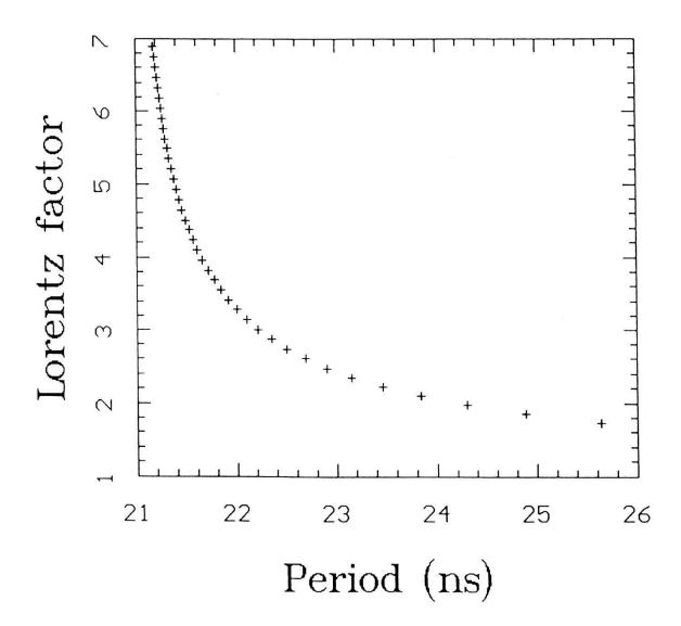
Figure 6: Theoretical prediction of Lorentz factor vs. period for muons in uniform circular motion in a uniform magnetic field, according to the Lorentz force law. The radius of circular motion is 1 m.
