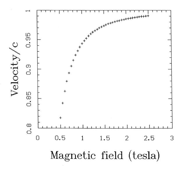
Figure 4: Theoretical prediction of v/c vs. magnetic field for muons in uniform circular motion in a uniform magnetic field, according to the Lorentz force law. The radius of circular motion is 1 m.
