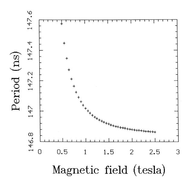
Figure 2: Theoretical prediction of period vs. magnetic field for muons in uniform circular motion in a uniform magnetic field, according to the Lorentz force law. The radius of circular motion is 7.0059 m.
