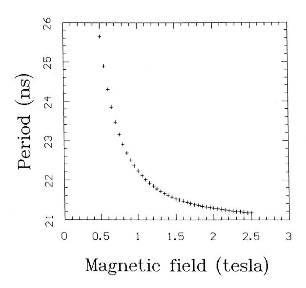
Figure 5: Theoretical prediction of period vs. magnetic field for muons in uniform circular motion in a uniform magnetic field, according to the Lorentz force law. The radius of circular motion is 1 m.
