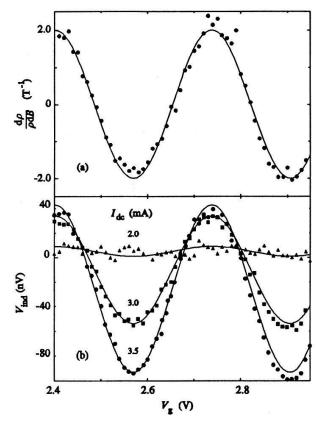
the induced voltage show the same periodicity as the SdH-oscillations in the longitudinal resistivity of the 2D EG.
