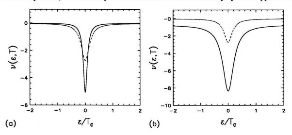
Figure 2: Leading corrections to Migdal's theory. The correction  $\nu(\epsilon, T)$  to the DOS is calculated for Einstein spectra with coupling constants  $\lambda_1=1.6$  ( $T_c/\Theta_D=0.18$ ), and  $\lambda_2=3.2$  ( $T_c/\Theta_D=0.29$ ). Results are presented for  $[\lambda_1, T/T_c=1.5, solid line in (a)], <math>[\lambda_1, T/T_c=1.8, dashed lines in (a) and (b)], and <math>[\lambda_2, T/T_c=1.8, solid line in (b)]$ .
