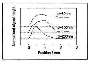
Figure 3 Linescans of 50, 100 and 200nm films. The scans were taken horizontally half way through the centre of the films, starting at the left hand edge. In each case  $T \approx T_C$  and  $I_b = 0.5$ mA.
