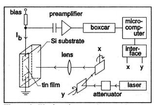
Figure 1 The imaging system
