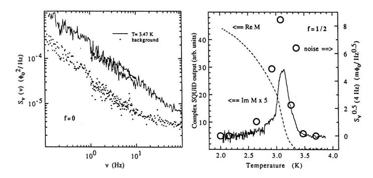
Figure 1: a) Spectral density of  $S_{\phi}(\nu, T=3.47)$  of a JJA (noise floor not substracted). b) Same quantity measured above the transition.
